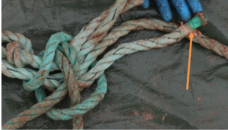
Figure 13. Clean/taped bitter end of Segment 2
