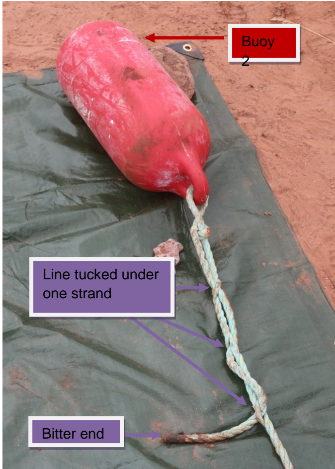
Figure 17. Segment 3- 1/2 in diameter 3-strand light blue-colored rope with yellow tracer, with Buoy 2 attached.
