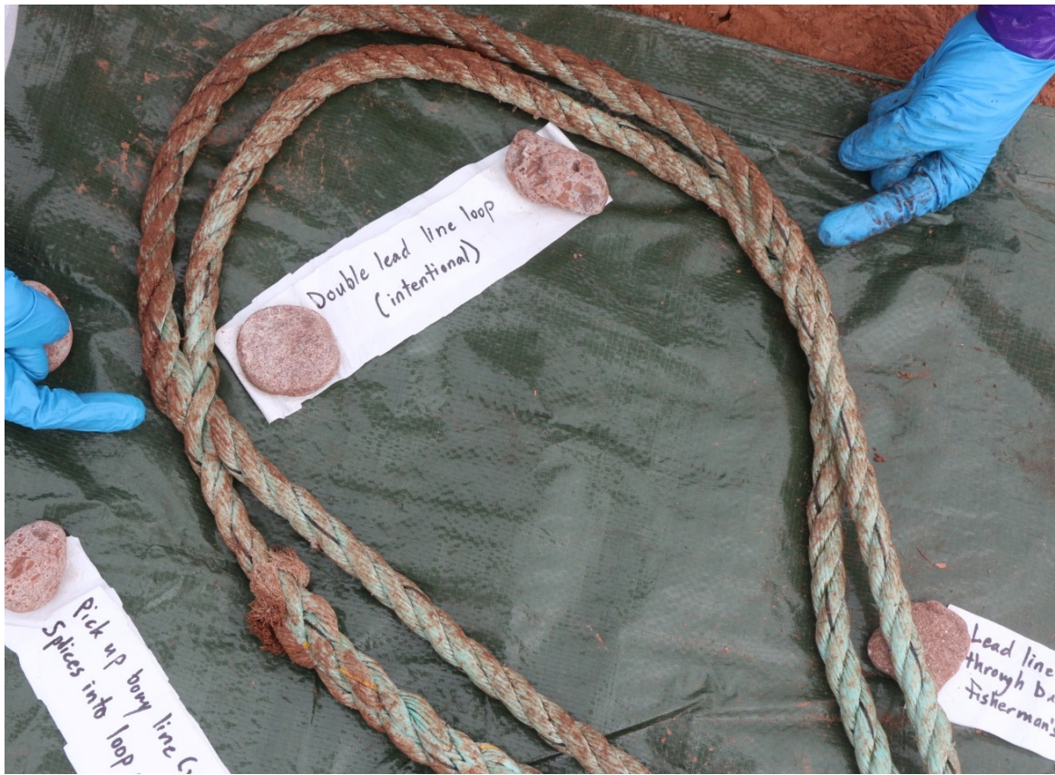
Figure 15. Lead line doubled back on itself and tucked under one strand in several places rather than knotted.
