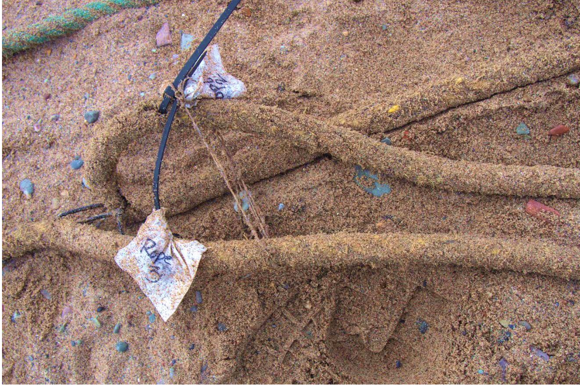
Figure 12. String tied to create a 1.22m loop in the yellow rope. Cable ties and labels added by examination team © Marine Animal Response Society.
